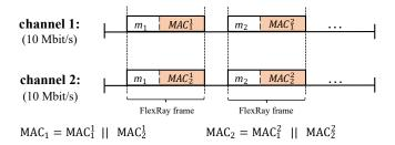
Figure 5: Transmission of cryptographic data under option 3: The message authentication code is split into two truncated parts, which are then separately sent over an individual channel.
