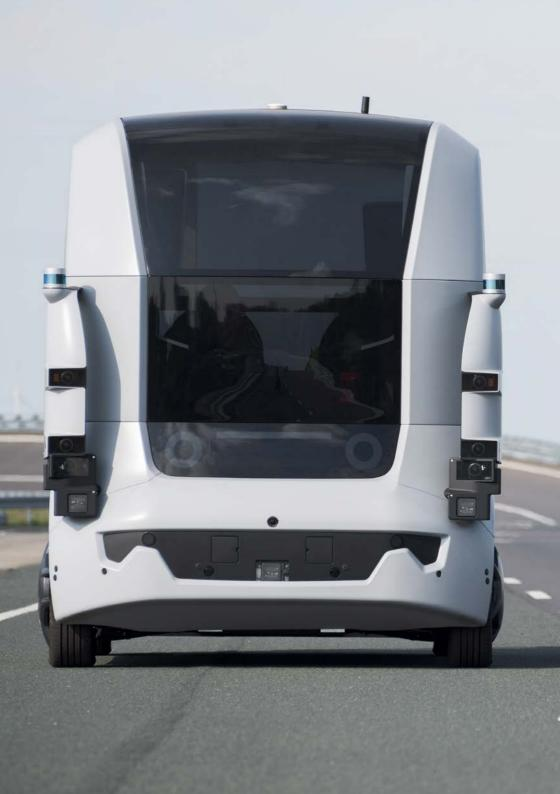
The UNICAR*agil* vehicles have four identically equipped sensor modules These modules are self-contained from the mechatronic as well as the functional point of view. Each sensor module comprises radar sensors, monocular cameras, a lidar sensor, a stereo camera system, an inertial measurement unit, and an associated computing unit for sensor data processing.
