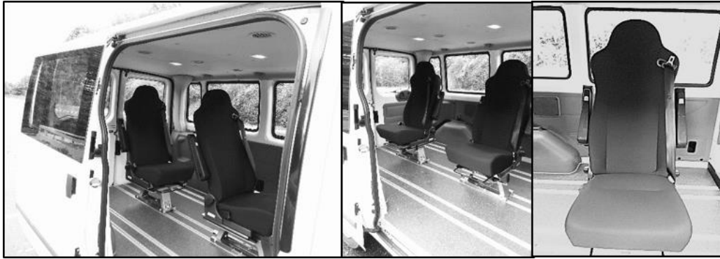
Fig. 4: Seats and exemplary seat configurations. Seats turned forward (1), 90° sideways (2) and full view of one seat (3)
