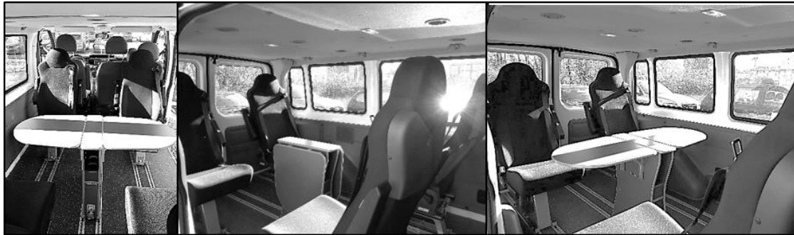
Fig. 8: Interior of the testing vehicle. Backward facing seats with table (1), all rear seats with folded table (2), forward facing seats with table (3)
