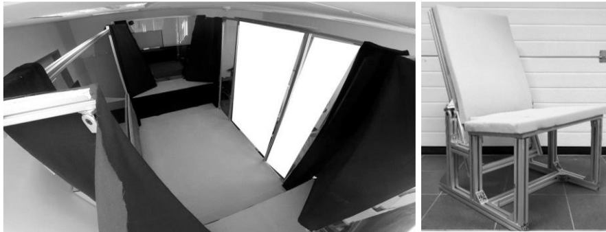
Fig. 1: Left: Inside of the autoSHUTTLE mock-up structure with usable floor area in the middle of 2740 mm * 1880 mm and three screens (front, left and rear view), right: the adjustable mock-up seat
